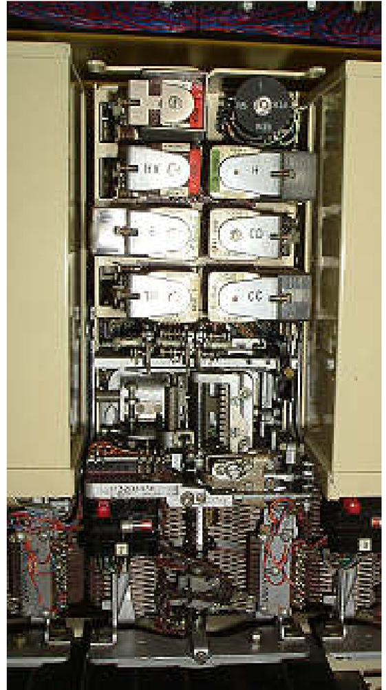
When the group selector is normal it returns a testing battery back to the linefinder, allotter and control relay set via the P wire. If the selector is in use (B relay operated), off normal (N2 springs operated), busied (red link removed from test springs 13 and 14), or the selector fuse has blown, the selector and its linefinder is busied to the allotter and control relays set.
